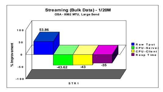
Figure 7: Streaming AWM – OSA jumbo frames, Large Send
