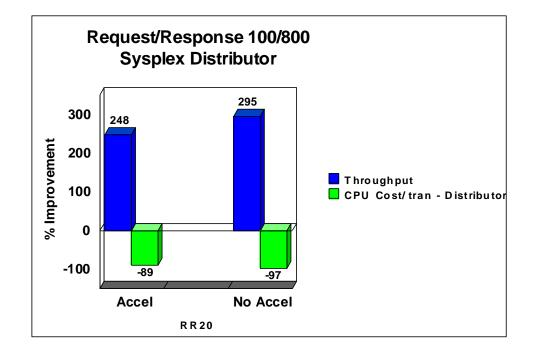
Figure 10: SMC-R with Sysplex Distributor performance
