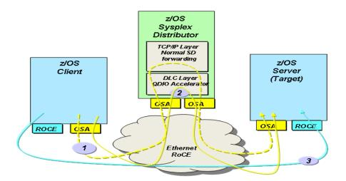
Figure 9: SMC-R with Sysplex Distributor
